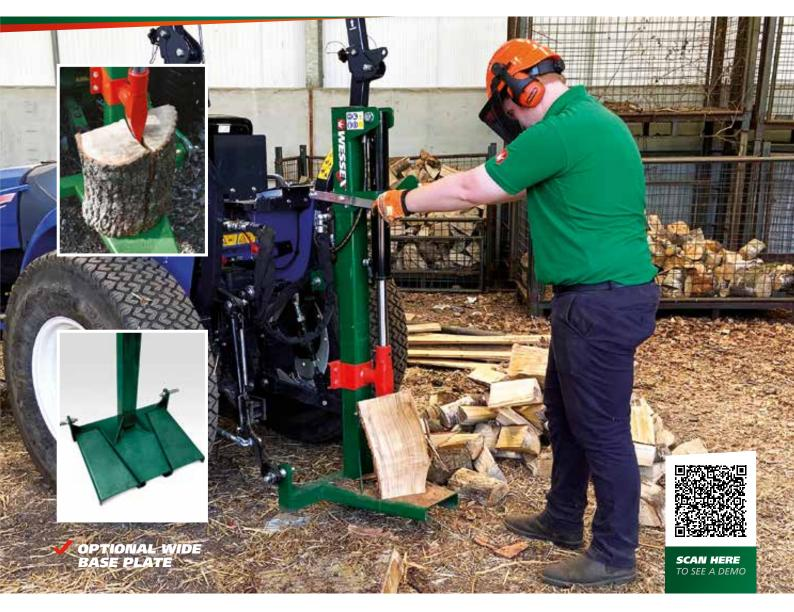
The Wessex **LS100 LOGSPLITTER** turns a chore into an enjoyable task! With up to 10 ton of splitting force\* at its disposal, the LS100 will effortlessly crack logs up to 18"/450mm in height.
