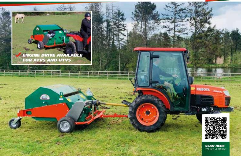
The Wessex MTX TRAILED COLLECTORS are available as a sweeper collector or a paddock cleaner in both PTO or engine driven versions for use behind a small tractor an ATV or UTV.
