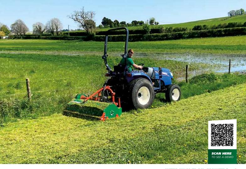
Engineered for unparalleled strength and durability, making the management of dense vegetation effortlessly efficient. Offered in 2.5m and 2.8m widths, these mowers feature hydraulic side shift for enhanced manoeuvrability.
