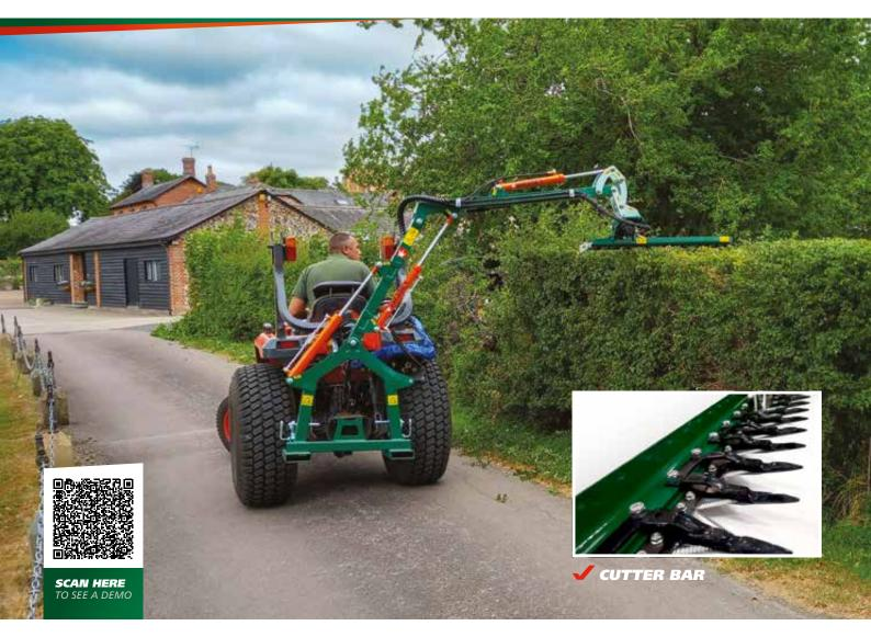
The Wessex **CHT-120** 1.2m hedge cutter is perfect for trimming small trees, hedges and pruning edges, and are ideal for compact tractors of 15hp and above. The model features a 1.2m cutter bar and comes complete with cable controls.
