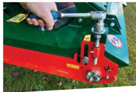
SIMPLE CUTTING HEIGHT ADJUSTMENT
