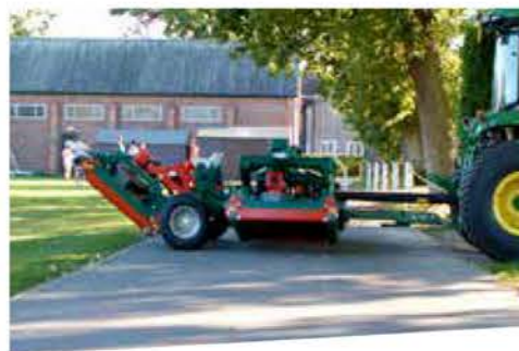
PRO-LIFT – ALLOWS SIMPLE PARTIAL DECK LIFT FOR CROSSING PATHS
