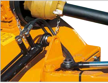
The arms rotating pivot has a self-lubricating bearing for minimal maintenance.
