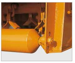
Adjustable rear roller - simple cutting height setting.
