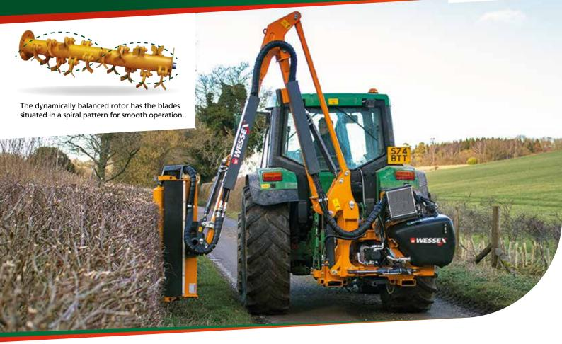
The **T500G AND TPE600** are the flagship models of the Wessex hedge cutting range. Both feature a 1.2m working width head with the option of various flail types for different applications.
