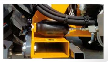
Optional lift float accumulator allows smooth operation with reduced bounce on the arm.
