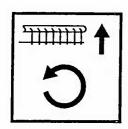
GB When scarifying, lift rotor before turning.
