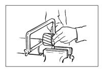
Round off all sharp edges and remove burrs. Grease sliding profiles.
