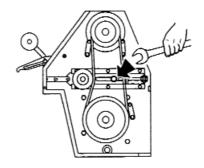
3. Tighten belts using adjusting screw and lock off.
