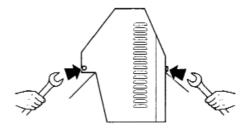
2. Loosen Jockey Pulley Bracket clamping bolt.
