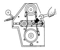
3. Tighten belts using adjusting screw and lock off.
