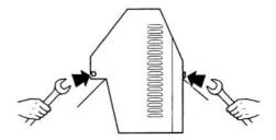
2. Loosen Jockey Pulley Bracket clamping bolt.
