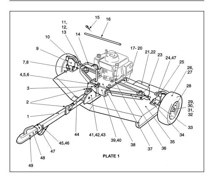
PARTS LIST - AR120 & AR150 MAINFRAME ASSEMBLY - PLATE 1
