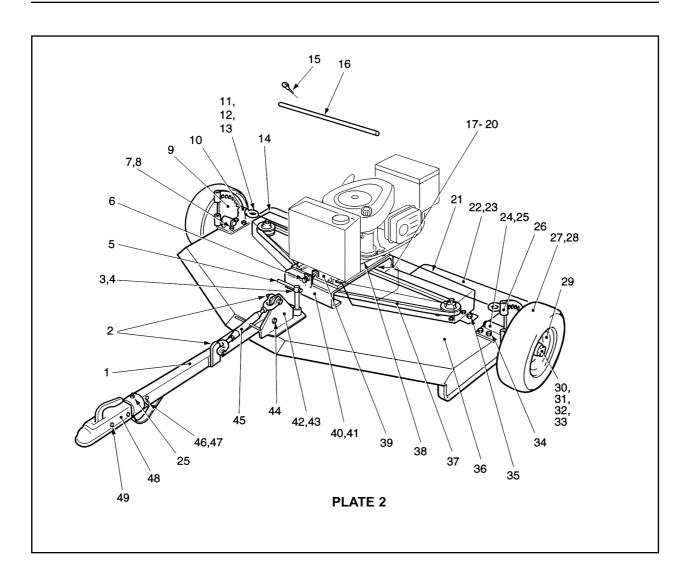
PARTS LIST - AR180 MAINFRAME ASSEMBLY - PLATE 2
