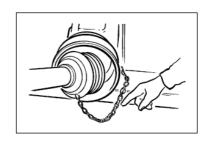
The PTO drive shaft must not be suspended from the chains!
