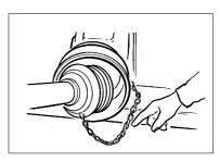
The PTO drive shaft must not be suspended from the chains!
