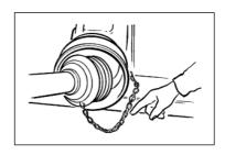
The PTO drive shaft must not be suspended from the chains!
