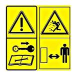
Disengage the PTO, turn off the tractor engine, remove the key and ensure that all rotaing parts have stopped before approaching the implement.
