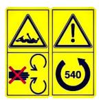
Operate only with 540 rpm PTO
