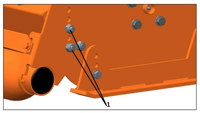
Depending on the different roller positions, it is possible to set four different cutting heights: 32-57-82 and 107 mm.
