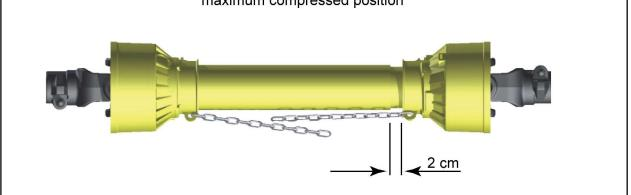
A driveshaft that is too long may cause structural damages to the tractor and machine. If the driveshaft is too long, it may be adapted by removing it and shortening the tubes according to the instructions provided by the Manufacturer in its use and maintenance manual.
