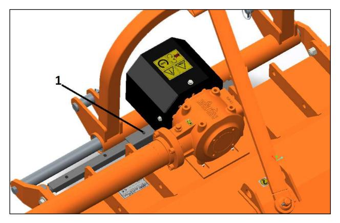
To check the correct belt tensioning of the side transmission, remove the safety cover of the belts by loosening the four bolts (1) that secure it to the frame (see picture):-
