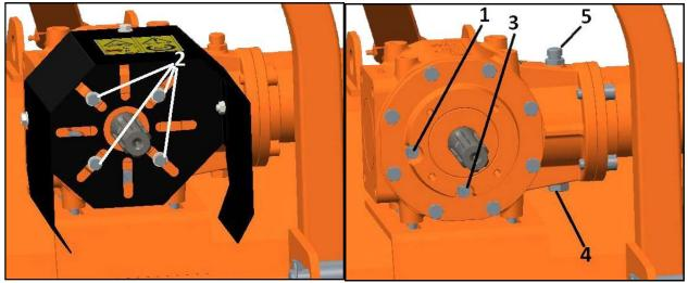
If the oil level is below the line of the level plug, it's necessary fill up oil till restore the correct level.
