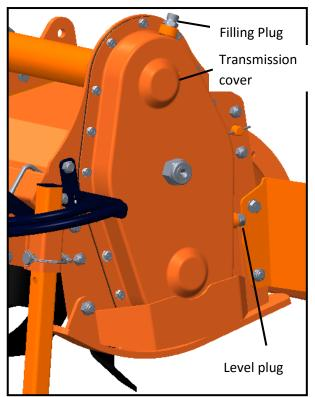
Check the oil level every 50 hours, making sure it reachs the level plug on the transmission cover. If the oil is below this level, fill up oil till restore the level.
