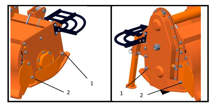
When finished, verify that both skids are at same level, and check if the front of the Cultivator is leveled to the back, when lowered to the ground. Adjust with the 3-point top link if necessary.
