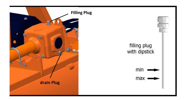
If the sign is below the minimum, fill up oil till restore the correct level. The oil change must be performed:
