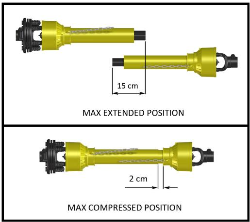
A driveshaft that is too long may cause structural damages to the tractor and machine. If the driveshaft is too long, it may be adapted by removing it and shortening the tubes according to the instructions provided by the manufacturer in its use and maintenance manual.
