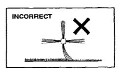
The brushes are not designed for scarifying or thatch removal, and damage to the brushes will quickly occur if it is used for this purpose.
