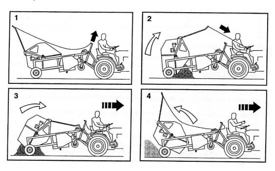
If possible the tip should be located so that the Sweeper can be driven right through, dumping the refuse on top of the previous load in order to consolidate it. Alternatively, the Sweeper can be reversed back onto the tip for the same effect.
