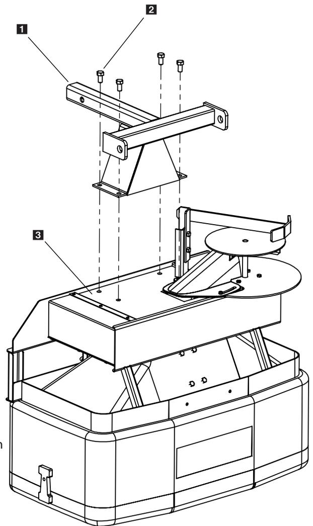
Note: Spreader shown in receiver mount configuration
