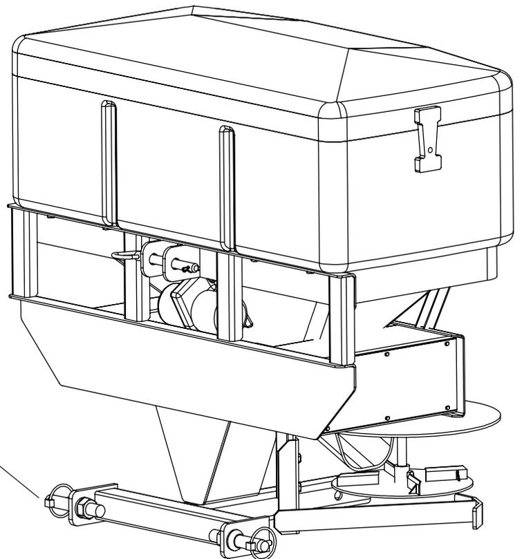
Note: Spreader shown in three point mount configuration
