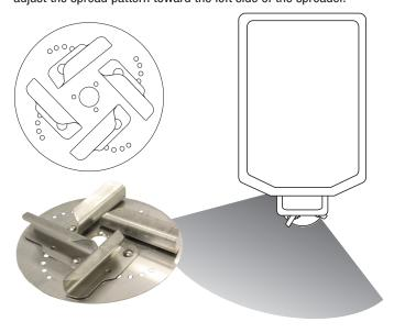
When looking down at the spinner, moving the fins counter-clockwise will adjust the spread pattern toward the right side of the spreader.
