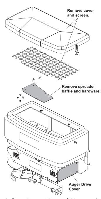
4. Remove the auger drive cover. Set the cover and all hardware aside. Remove all four bolts that hold the motor and gearbox to the frame. Slide the motor and gearbox out of the frame. Once the gearbox is removed, the auger can be removed.
