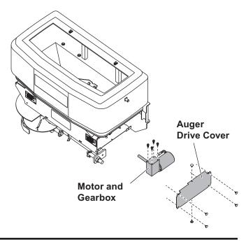
3. Position the auger so that the auger and auger tube sit unobstructed in the hopper tub. Once the tube is positioned, mark the mounting holes on the auger gearbox side position.
