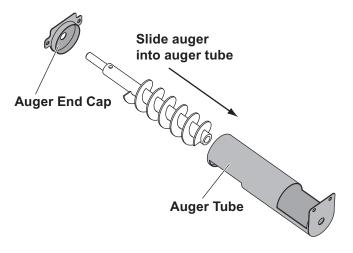
2. Install the motor and gearbox back into the frame. The gearbox output shaft will slide into the auger as before. Attach the gearbox mounting hardware to the hopper frame and tighten fasteners finger tight. Make sure the auger set screw is on the flat of the gearbox output shaft and tighten it down. Once the auger set screw is fully tightened, tighten the gearbox mount bolts according to the torque chart.
