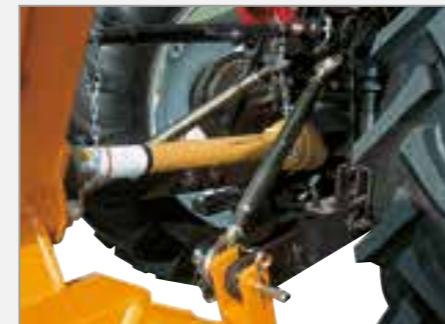
TRACTOR STABILIZERS MAINTAIN RIGIDITY ON THE TRACTOR.
