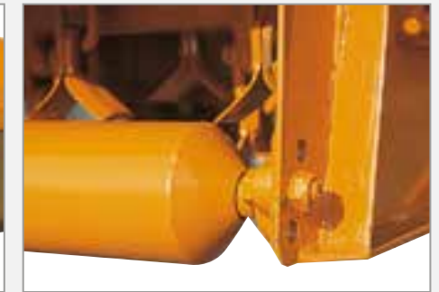
ADJUSTABLE REAR ROLLER - SIMPLE CUTTING HEIGHT SETTING.
